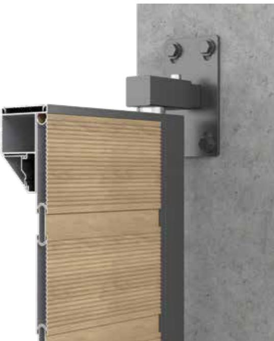
Detailed views of the sash and grooved profiles, along with the pivot axis profile with INOX 316 PIN able to hold 250 kg each. Maximum single door sash is close to 4m<sup>2</sup> withstanding a maximum wind load of 2KPa.
